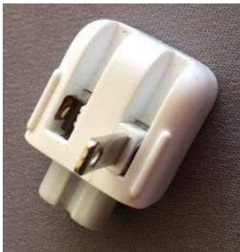
Power Adapter With Broken Blade
