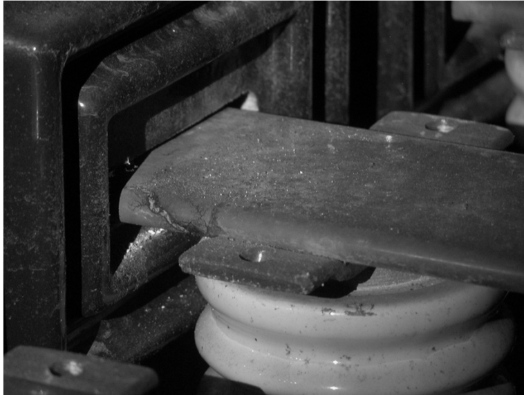
Tracking that led to full discharge / failure
