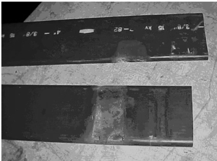
Insulation damage detected by on-line Partial Discharge monitoring
