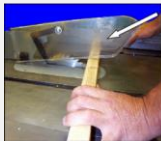
Circular table saw self-adjusting guard
