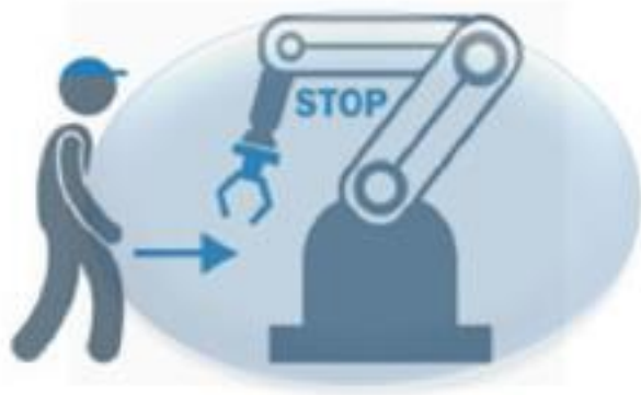
Type 1 – safety rated monitoring stop (SRMS)
