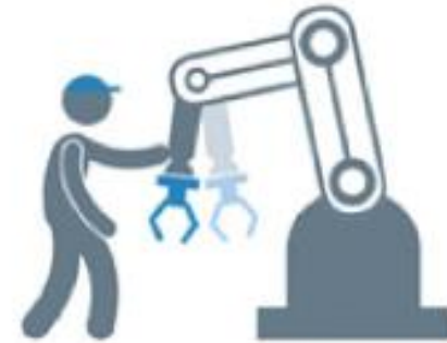
Type 3 – speed and separation monitoring (SSM)
