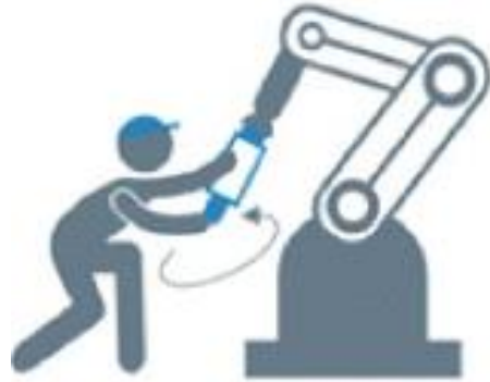
Type 1 – safety rated monitoring stop (SRMS)
