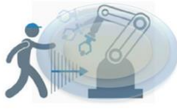
Type 3 – speed and separation monitoring (SSM)
