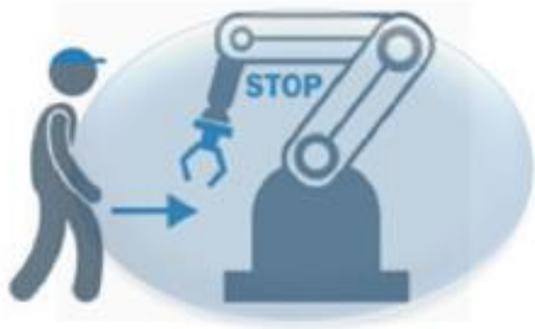
Type 1 – safety rated monitoring stop (SRMS)
