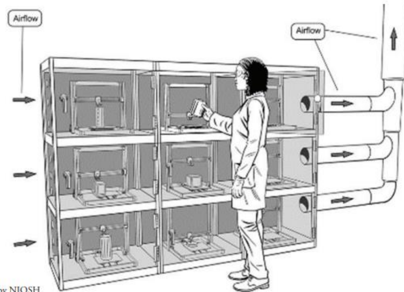
Figure 10. Drawing of a ventilated Plexiglas® enclosure surrounding a bank of 3D printers.
