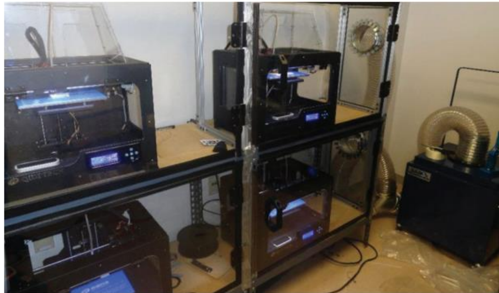
Figure 10. Drawing of a ventilated Plexiglas® enclosure surrounding a bank of 3D printers.
